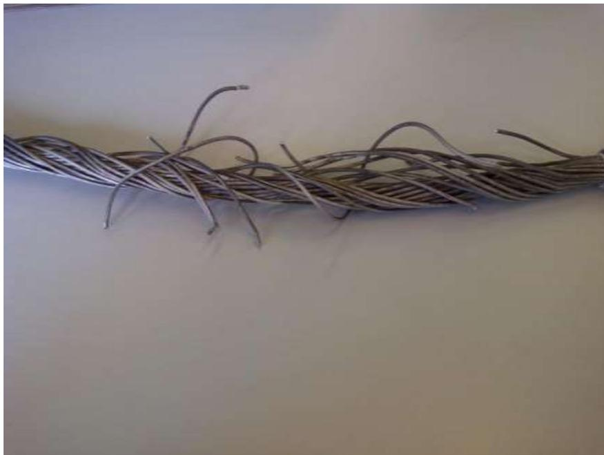
Figure 12 – 18L - Conductor damage removed in 2012
