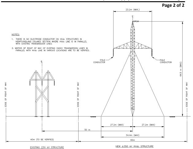
±350 kV HVdc Right of Way parallel with existing 230 kV line
