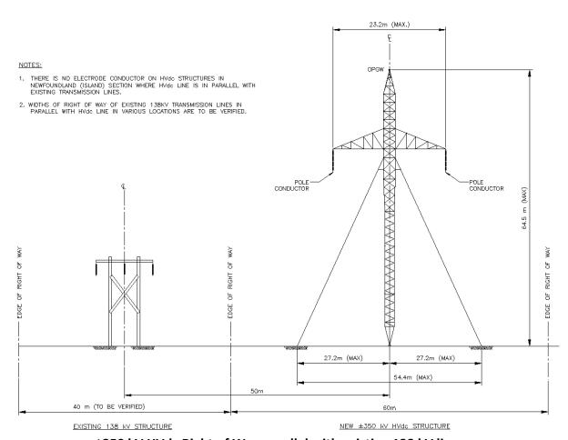
±350 kV HVdc Right of Way parallel with existing 138 kV line
