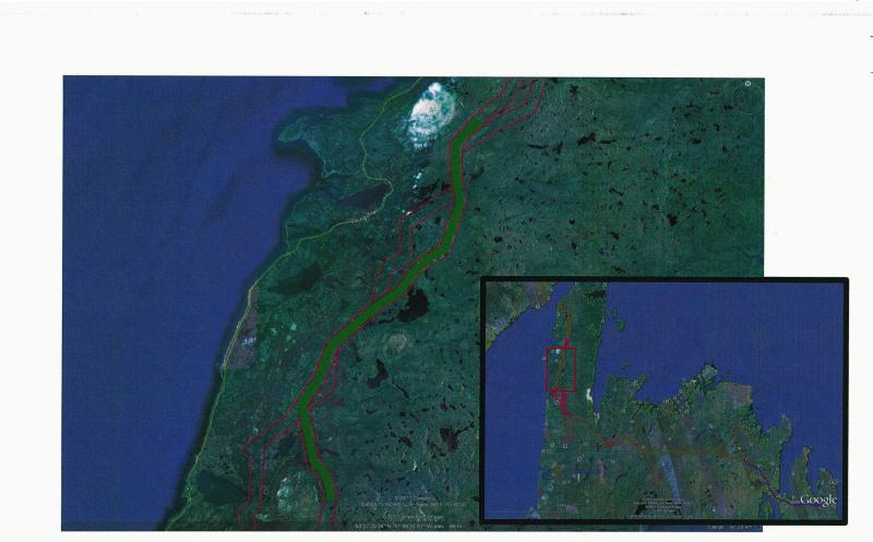
**Zone 6 – Northern Peninsula** Average Meteorological Loading Zone Maximum Ice: 50 mm (Glaze), Maximum Wind: 120 km/h, Combined Ice and Wind: 25 mm (Glaze) and 60 km/h
