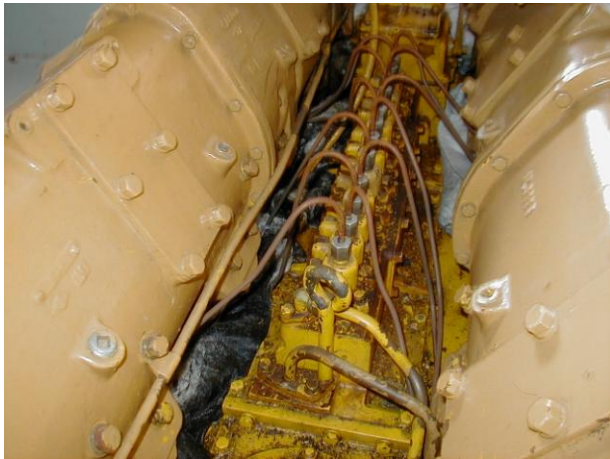
Fuel Leaks in the Engine Vee
