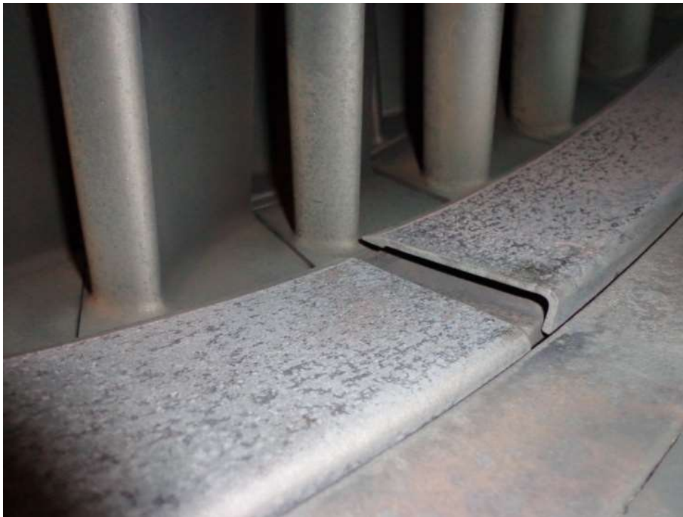
Figure 4 – Retaining Ring Distortion
