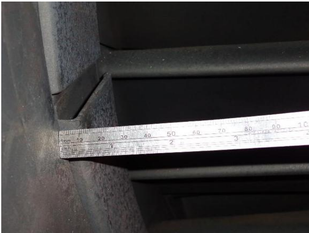
Fig 3 Protrusion of stator shroud
