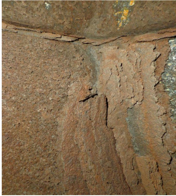
Fig 1 Corrosion in exhaust system.
