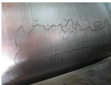
Figure 7 - Turbine guide bearing showing filiform corrosion. Depth of defect is about 0.0005"
