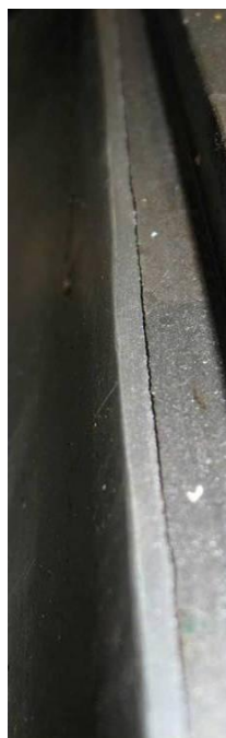
Figure 9 – Delaminating of Babbitt
