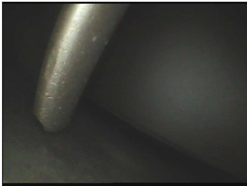
Fig 2 Blade impact damage and pitting
