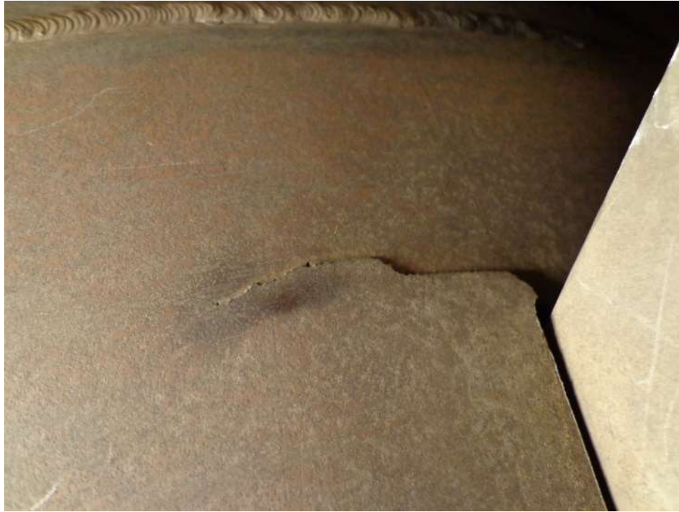
Figure 3 – Crack in Power Turbine Inlet Duct
