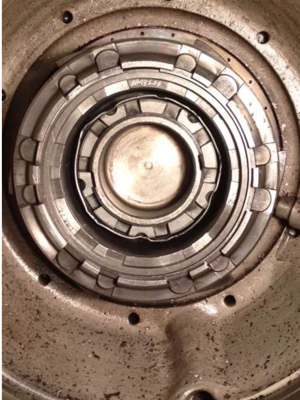
Figure 4 – Damaged Front Bearing
