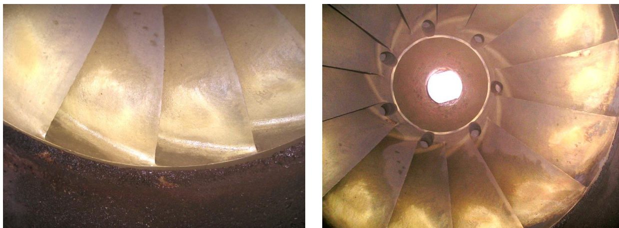
Figure 7 – 2007 Inspection of Low Pressure Side of G1 Runner showing Belzona Erosion and Cavitation
