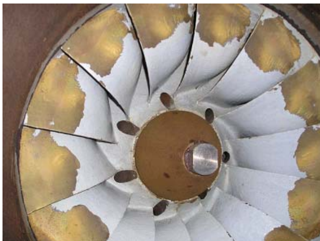
Figure 2-Low pressure side showing loss of belzona coating
