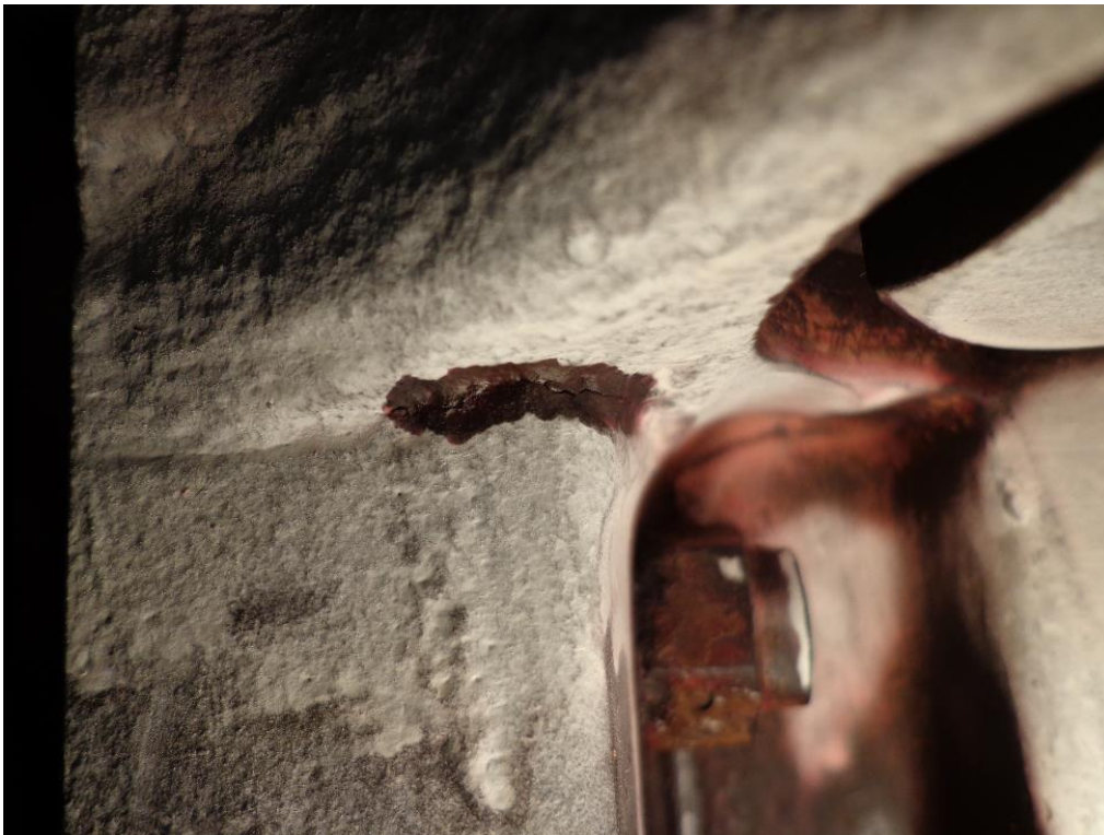
Fig 4 Crack in pressure casing
