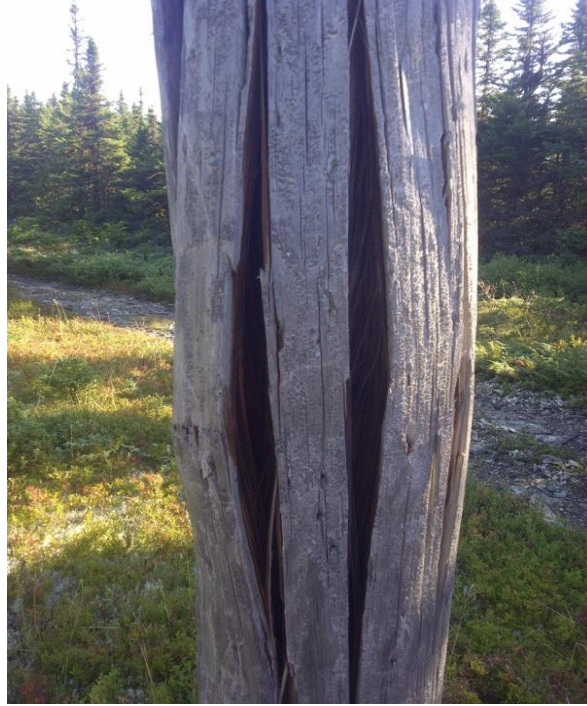
Failed Transmission Line Pole, 35 L, St. John's
