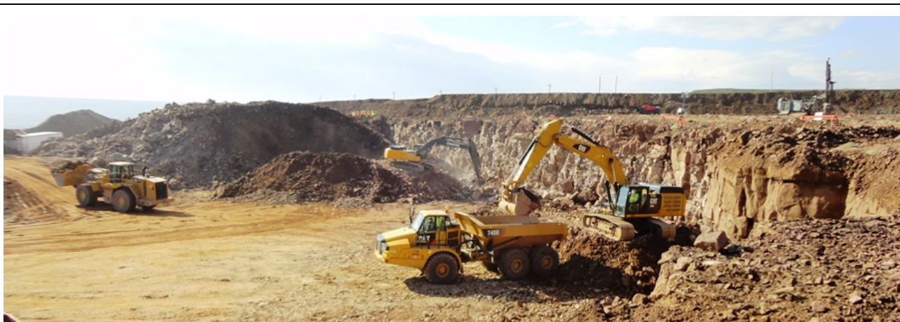
Photo 4.1: Forteau quarry. Principal quarry face on the right side of the photograph. Note stockpile of unprocessed rockfill in left background. (July 15, 2014)
