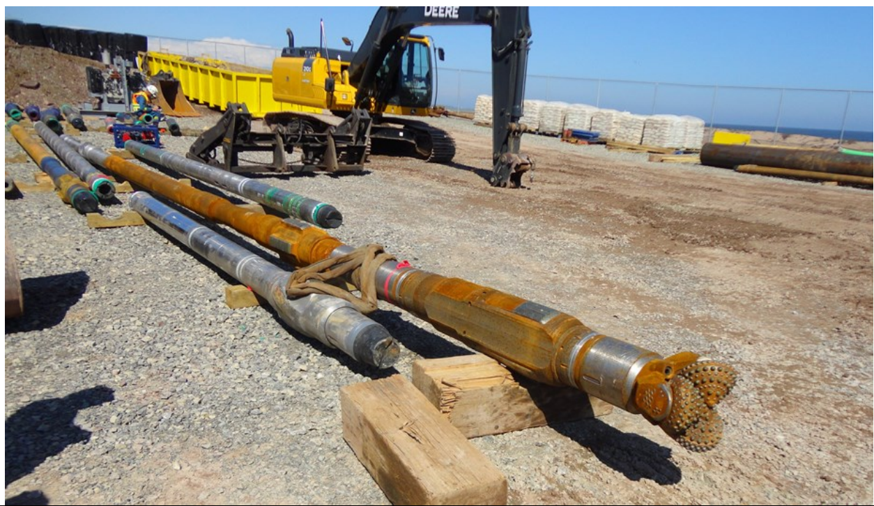
Photo 2.5: Forteau Directional Drilling. Drill bit and lower non-magnetic drill string components. (July 15, 2014)
