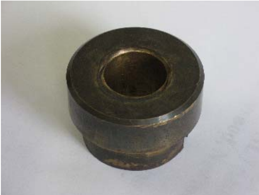
Figure 10.1 Shaft Bushing Worn
