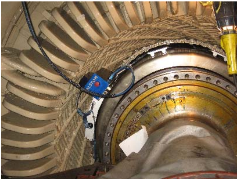
Figure 8.2 DIRIS Unit Installed in Air Gap
