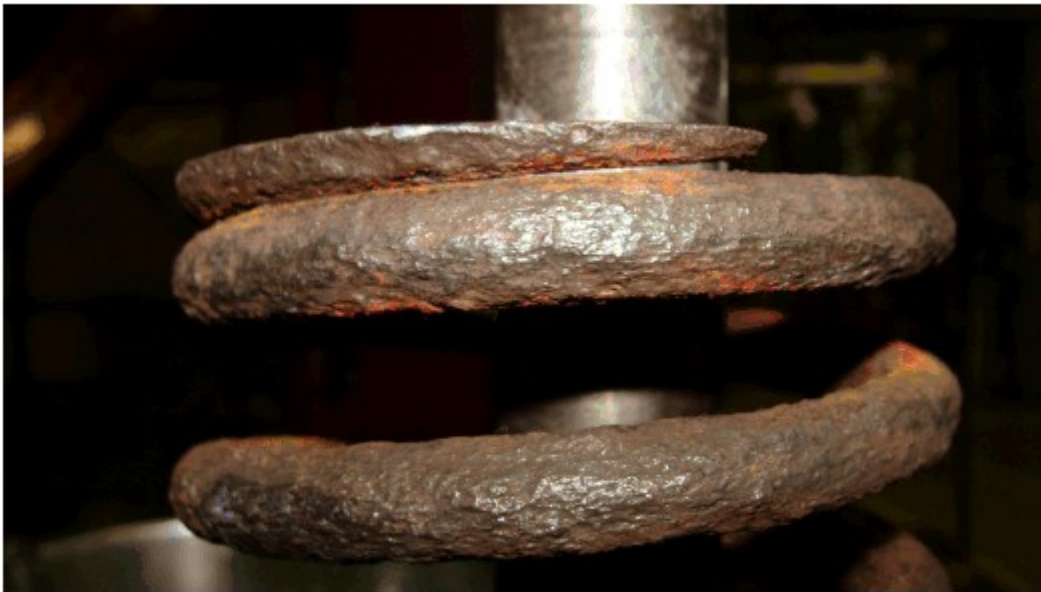
Typical rust conditions of springs in the NRV air operated actuators
