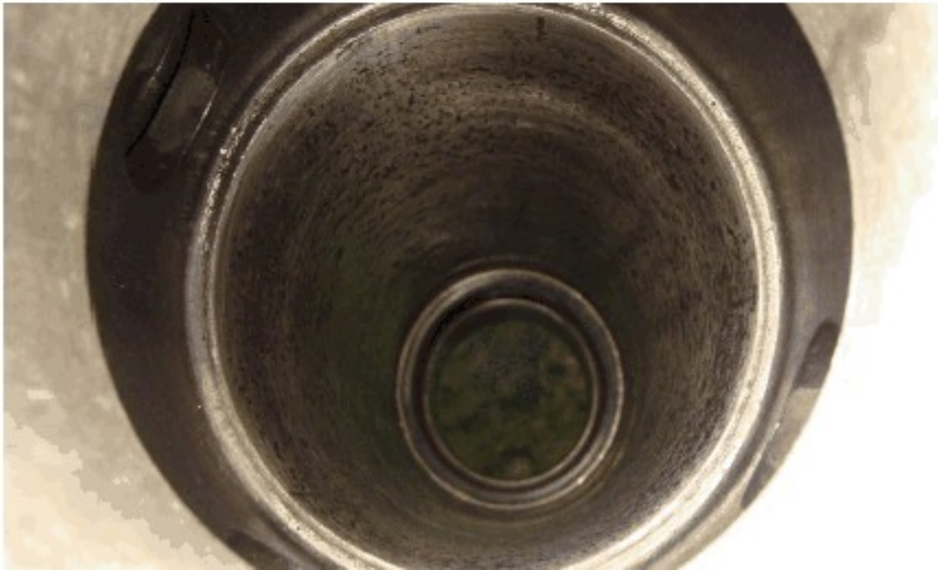
Blue Chk. MSV Stem Seal Visual shows good blue contact
