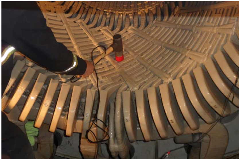
Figure 6 Impacting point for the NDE global modal analysis
