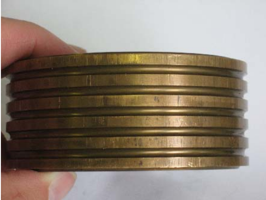
Figure 10.2 Scoring and wear of piston
