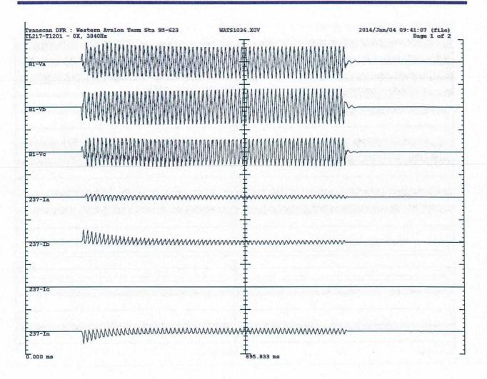
Figure 3: Circuit Breaker B1L37 at Western Avalon closes on two phases only 9:41 Jan. 4, 2014
