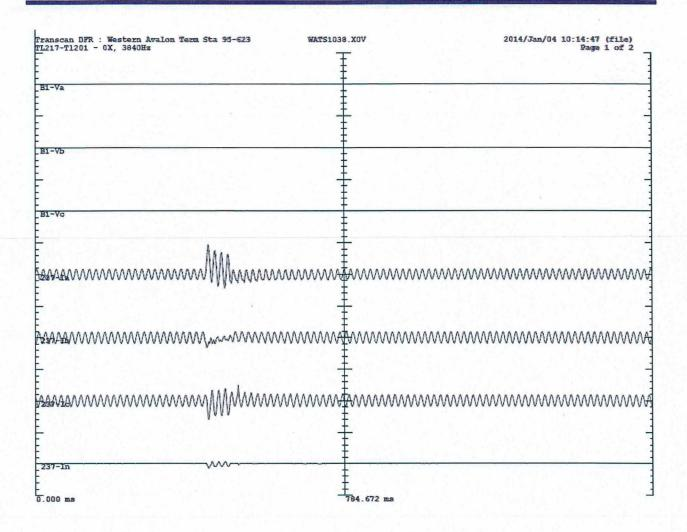
Figure 4: Holyrood generator transformer T1 is energized 10:14:43 Jan. 4, 2014
