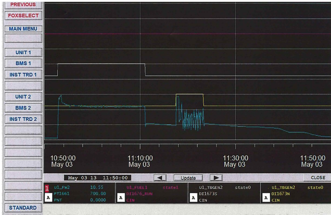
Figure 4: Test of DC Pump when coupled to AC South motor. Note that a test of AC pump South (white) provides normal and stable lube oil pressure (blue). When the AC North motor (yellow) is ran while coupled to the DC pump a similar cyclic pattern is exhibited as when DC motor and pump are ran together.
