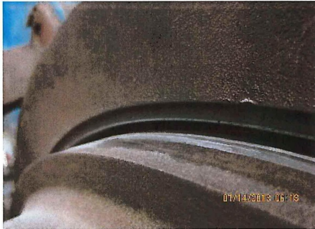
Figure 3 Bearing #4 – upper oil deflector clearance
