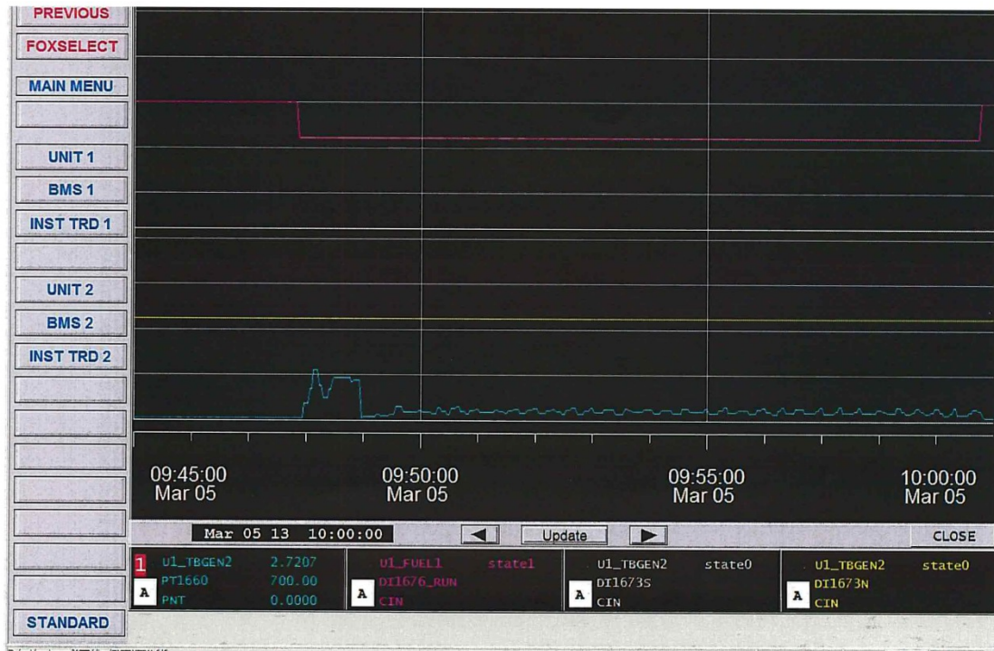
Figure 2: DC lube oil pump test from March 5, 2013. Note the falling magenta line indicates starting of the DC lube oil pump. There is an increase in pressure (blue) for a short time before pressure crashes and cycles
