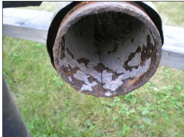
This is the same 4-inch section of pipe as in picture #1 after it has been cleaned. The corrosion pitting is on the order of 0.080-0.110 inch deep. Picture taken in August 2006.
