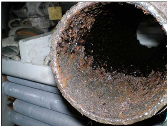
A fouled 4-inch section of surface air cooler piping, removed from service in 2006 due to severe corrosion. Picture taken in August 2006.
