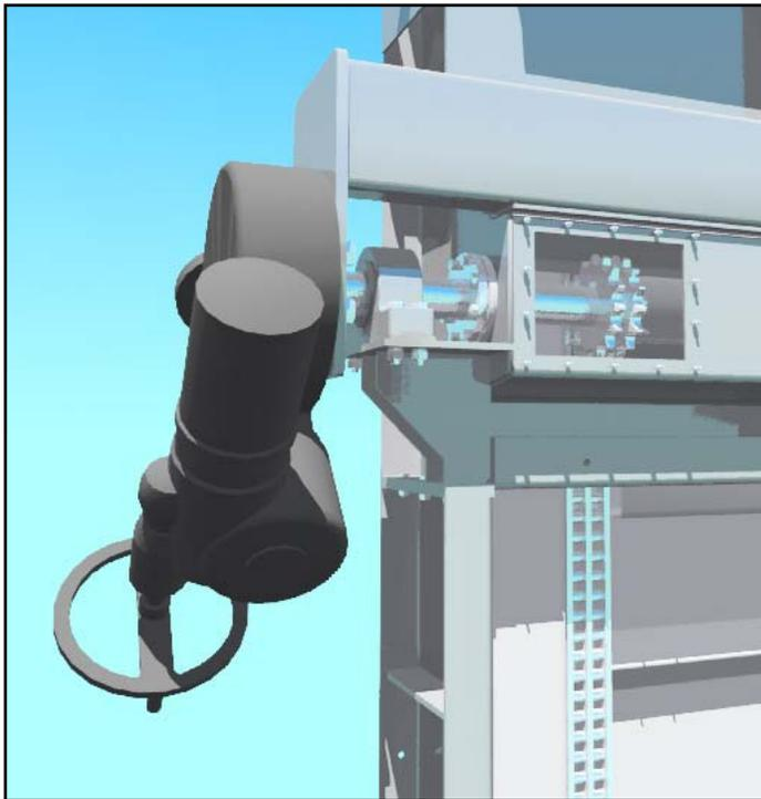
The drive system consists of two rigid pin racks attached to the blade, a drive pinion on each rack, supporting bearings with shaft seal assemblies, and an electric actuator with self-locking gearbox mounted on suitable brackets.
