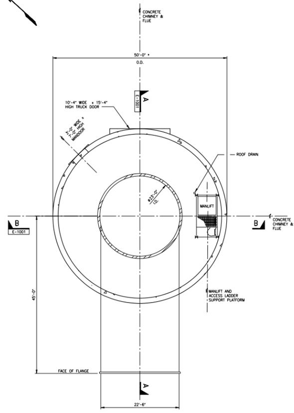
PLAN - CONCRETE CHIMNEY & FLUE
