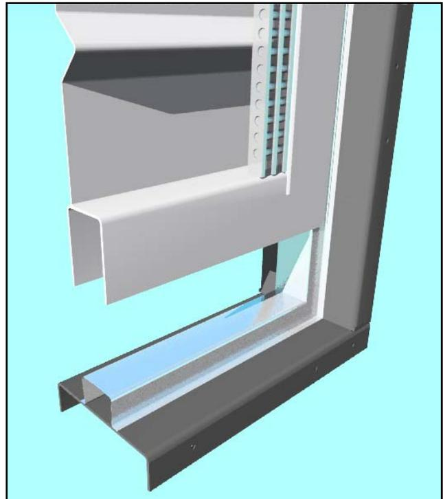
This blade design offers other benefits over the conventional solid plate blade design. Since the design uses only suitably reinforced thin membrane, it weighs only a fraction of what a
