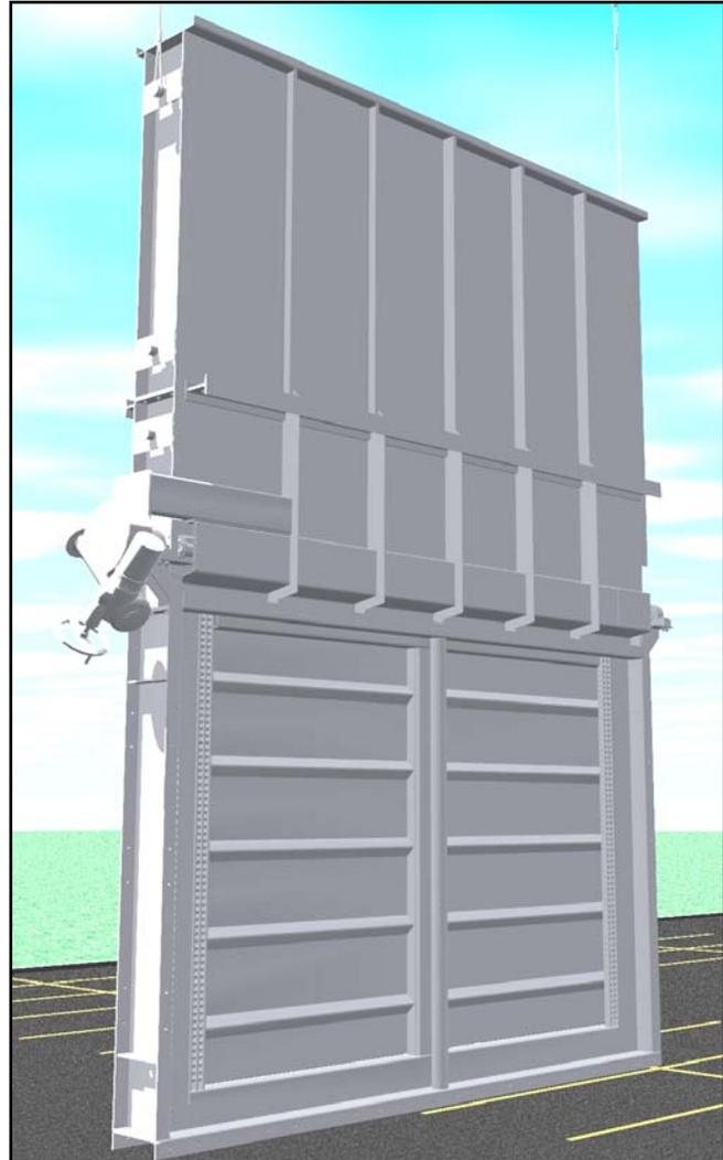
The frames are self-supporting structural members that do not require any external bracing or support. The frames are rigid and capable of withstanding loads generated under operating conditions without distortion that could affect the operation or sealing characteristics of the damper.
