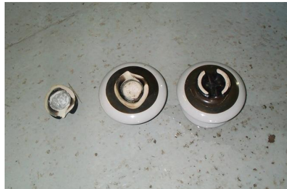
Figure 7: Broken Insulator Removed From Service
