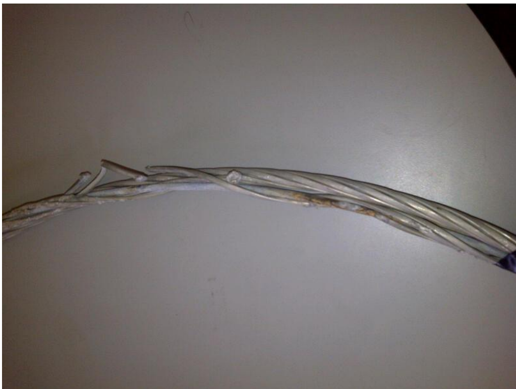
Figure 4 – 110L – Damaged conductor removed from 110L in December 2011
