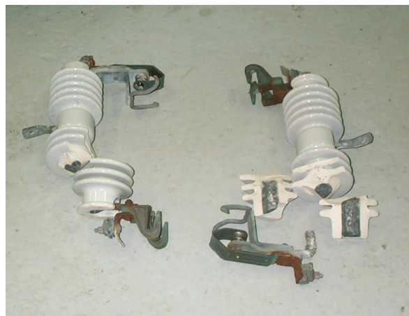
Figure 12: Two Broken Porcelain Cutouts Removed From Service
