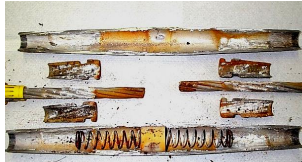
Figure 10: Disassembled Automatic Sleeve Showing Corrosion
