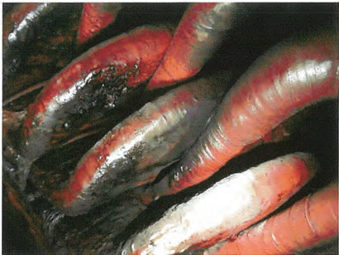
Resin present on knuckles is an indication of overheating.
