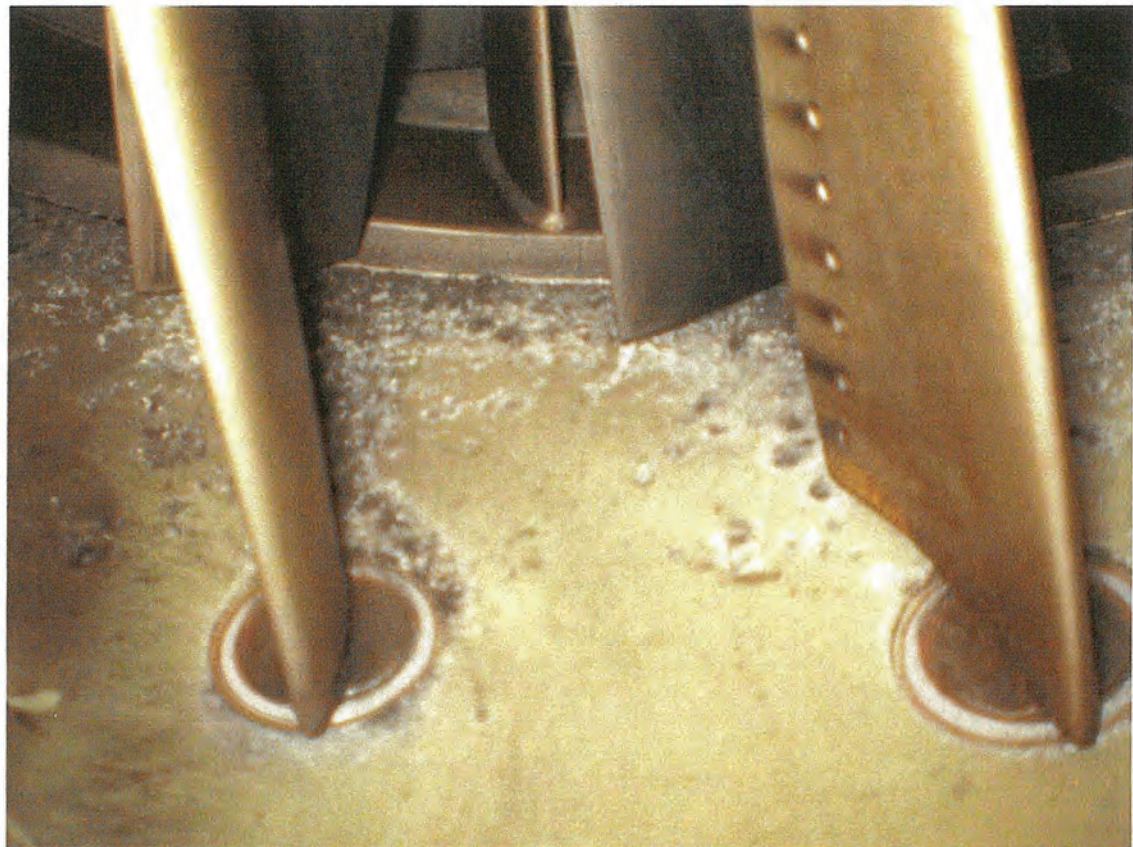
Light to medium corrosion noted to inner surface of the front bearing housing
