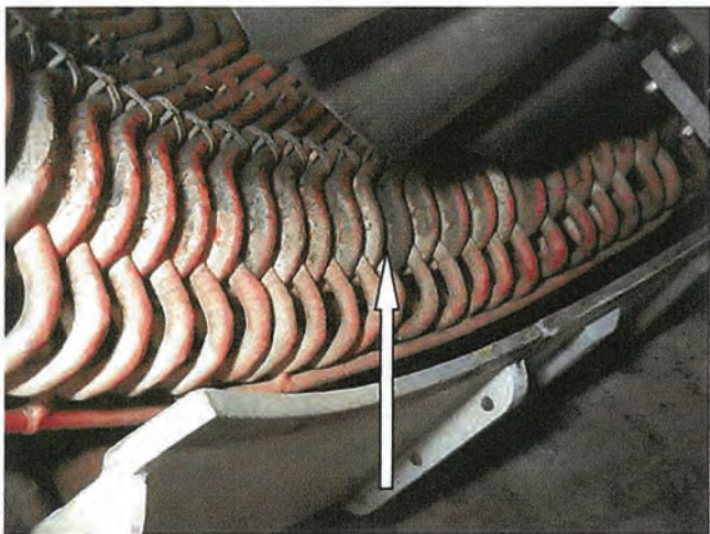
Discoloration heating pattern on some coils.
