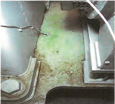
Leakage on bearing foundation
