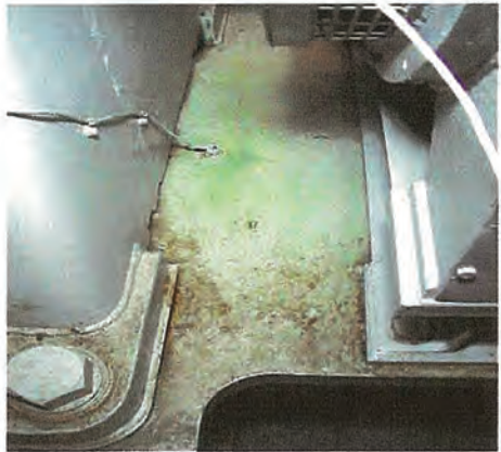
Leakage on bearing foundation
