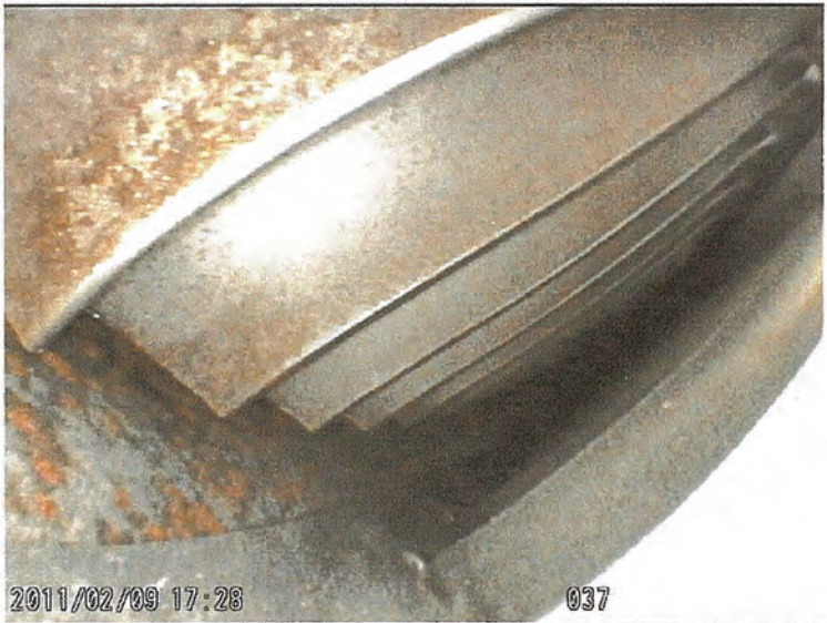
Photo 5. Showing corrosion of the nozzle blade track and on Rotor blade.
