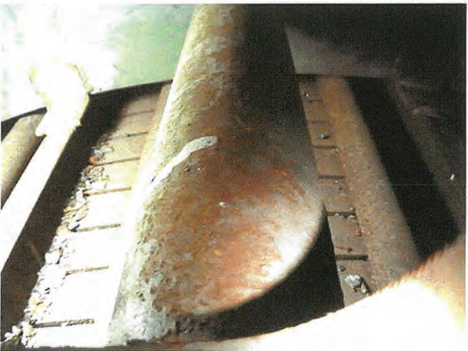
Rust flakes present on top stator core from exhaust/ventilation.
