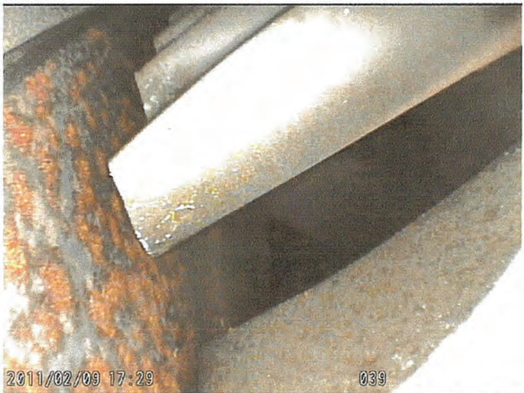
Photo 6. Showing corrosion of the nozzle blade track and on Rotor blade.
