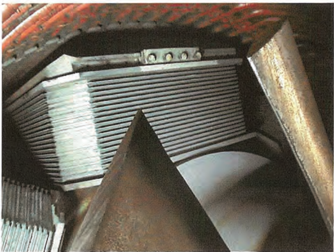
Rub mark on fan blade edge showing previous contact with fan cover.
