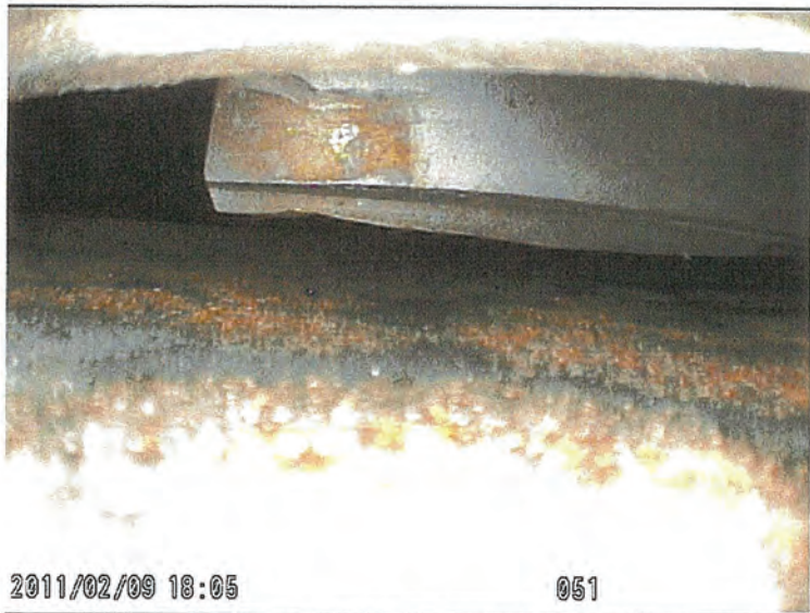
Photo 7. Showing worn blade tips.
