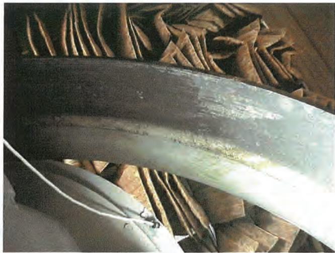
Wear marks on fan cover showing previous blade contact
