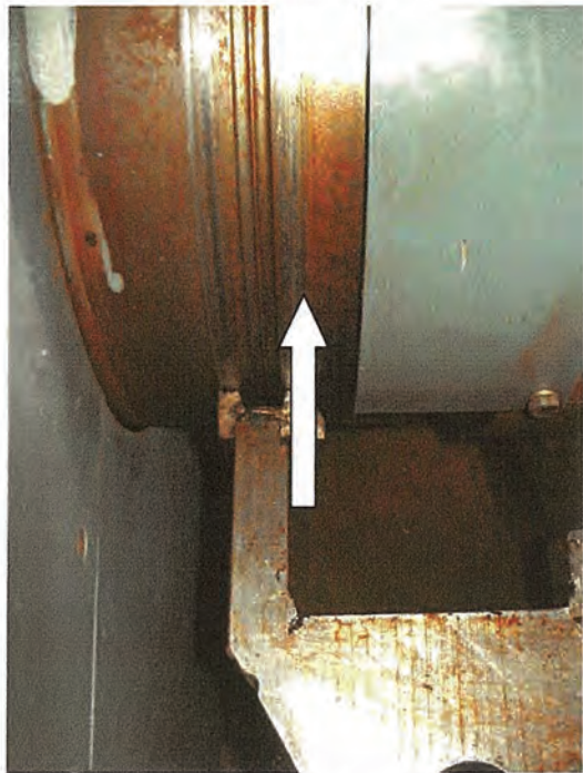
Outboard labyrinth seal and shaft seal (grooves wear marks)
