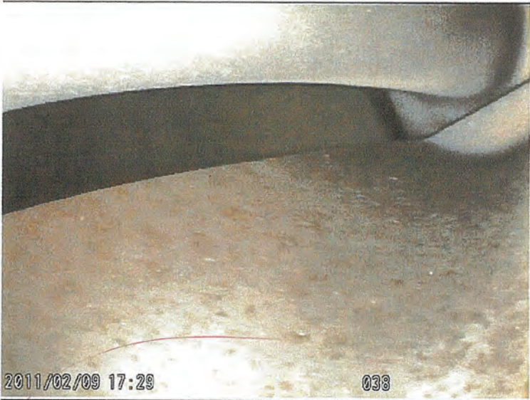
Photo 9. Showing corrosion on blades.
