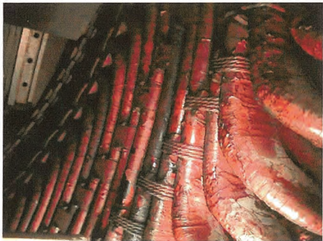
Dry brittle flaking insulation on coils
