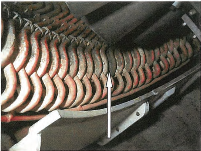
Discoloration heating pattern on some coils.
