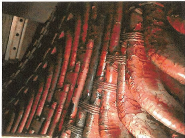
Dry brittle flaking insulation on coils
