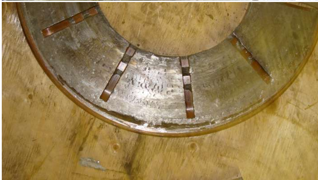
Active thrust pad condition
