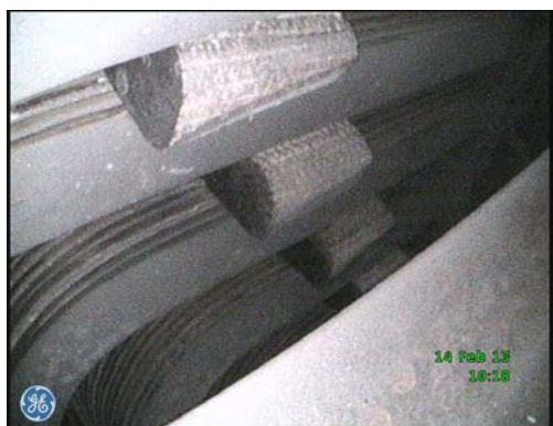
Coil wedges in position, heavy black dust present.
