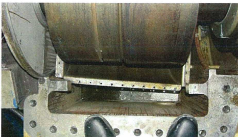
Lower half coupling guard lying in bottom of sump and Babbitt in bottom of sump
