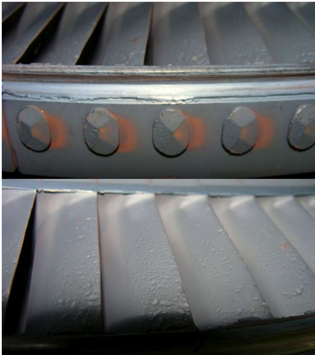
Row 3 blade root rub and inlet condition
