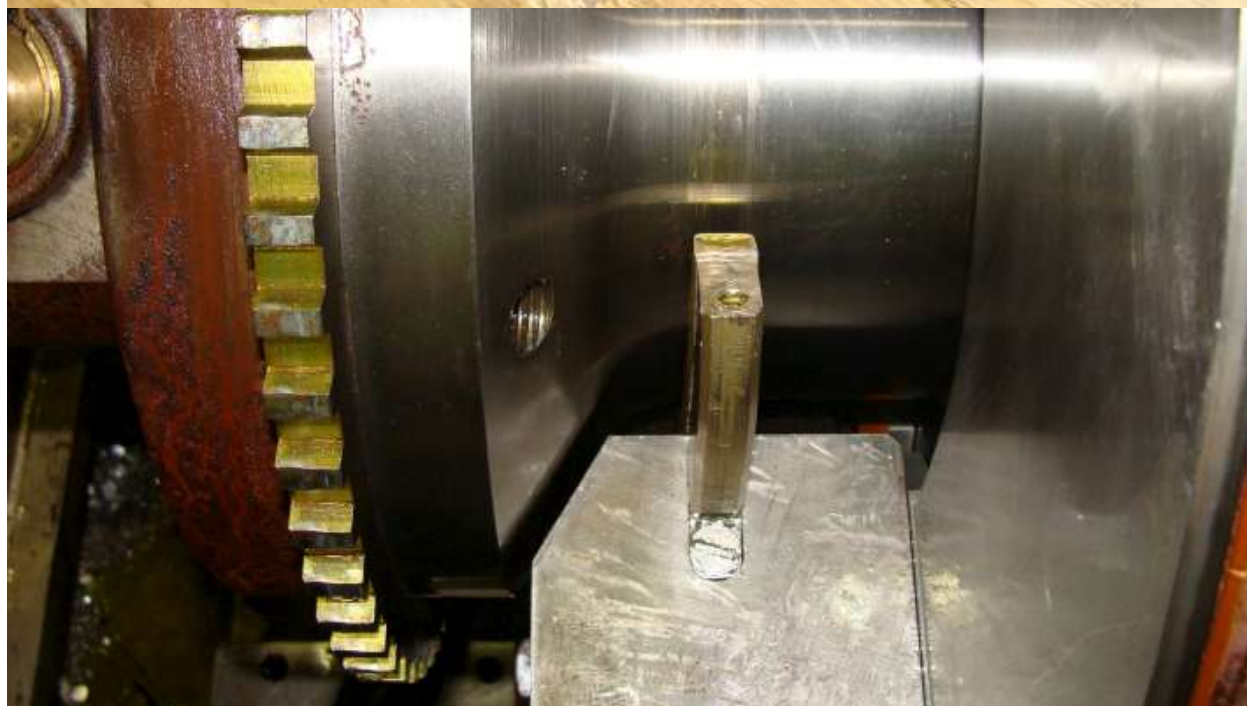
Seal ring rolled, keeper damaged
