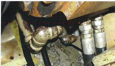
Babbitt in Front Standard below Thrust Cage
