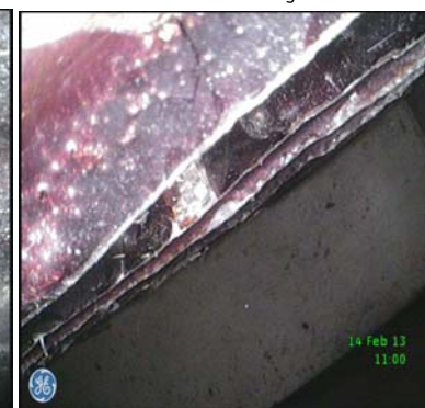
Blackened inter turn insulation
