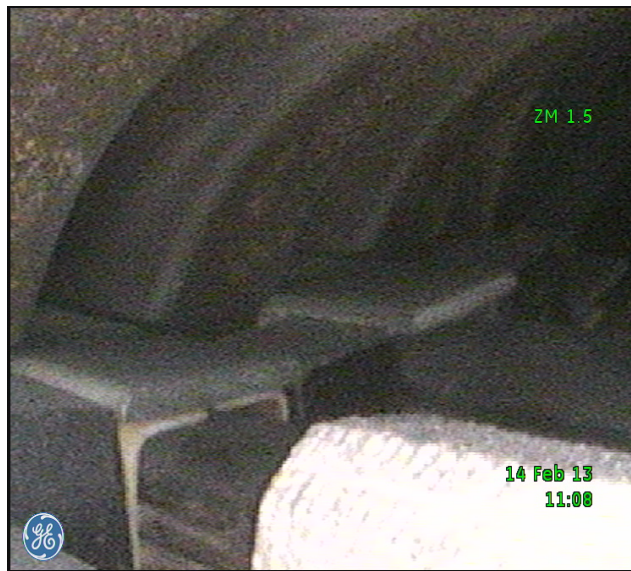
Slot exit insulation in position but contaminated throughout.
