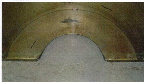
Upper half coupling guard showing rub in bore at horizontal joint area – one axial rub
