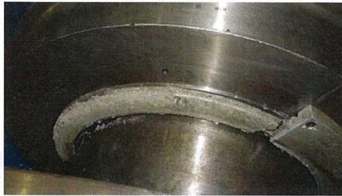
T3 Bearing U/H with upper bolt on seal removed – notice Babbitt
