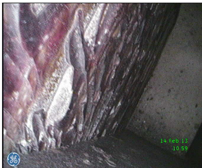
Seems resin has run down the coils & been contaminated. Note debris at base of coils.
