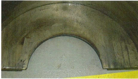
Lower Half coupling guard showing rub in bore
