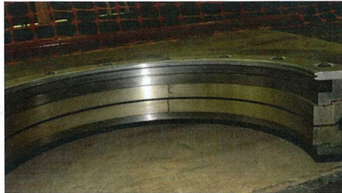
TE Hydrogen Seal Casing U/H removed – upper gas side oil seal heavy rub
