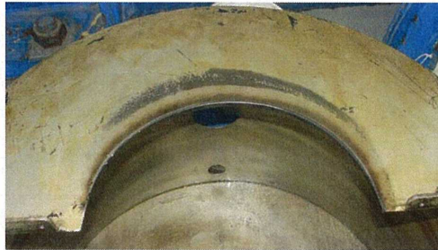
Lower half coupling guard with rubbing in bore
