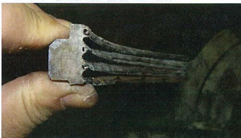
R1 Packing Ring - damaged
