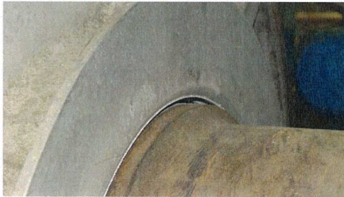
T3 Outer oil deflector prior to removal
