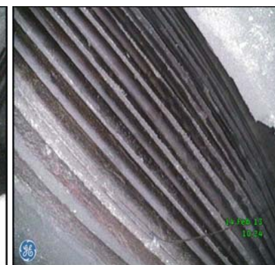
Interturn insulation has seen high heat levels
