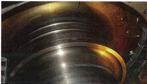
T5 inner oil Deflector shaft area showing rub
