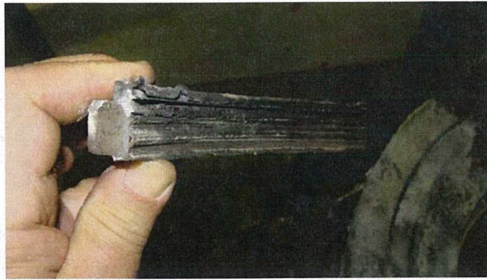
R1 Packing Ring Damage
