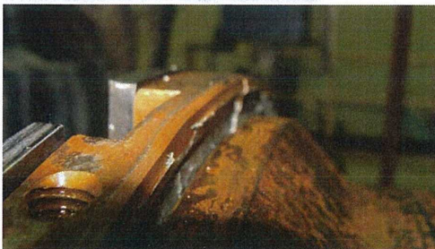
Thrust Active Side – Thrust Runner Rubbed into Thrust Plate
