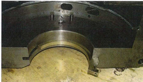
Thrust Cover U/H Rolled Oil Seal ring and broken screw
