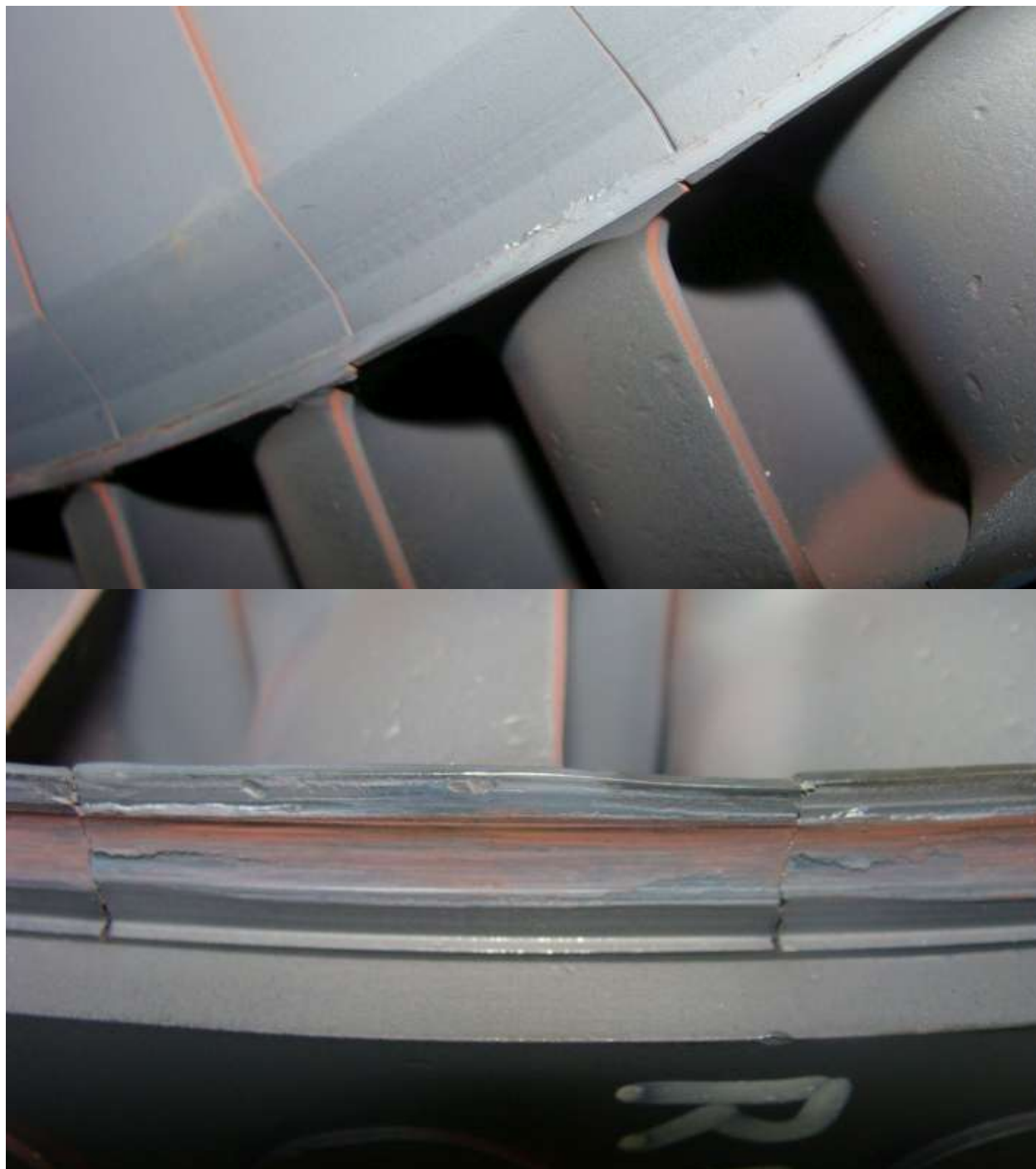
Stage 1 blade integral cover rub
