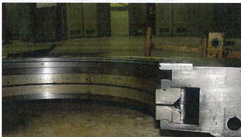
CE H2 Seal Casing U/H hard rub on Gas side Oil Deflector
