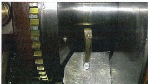
Thrust Bearing oil seal ring – rolled up and broken retainer screw
