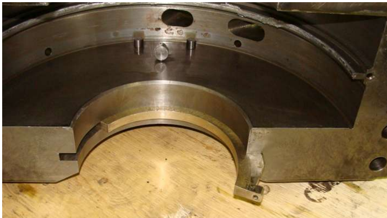
Seal ring rolled and damaged
