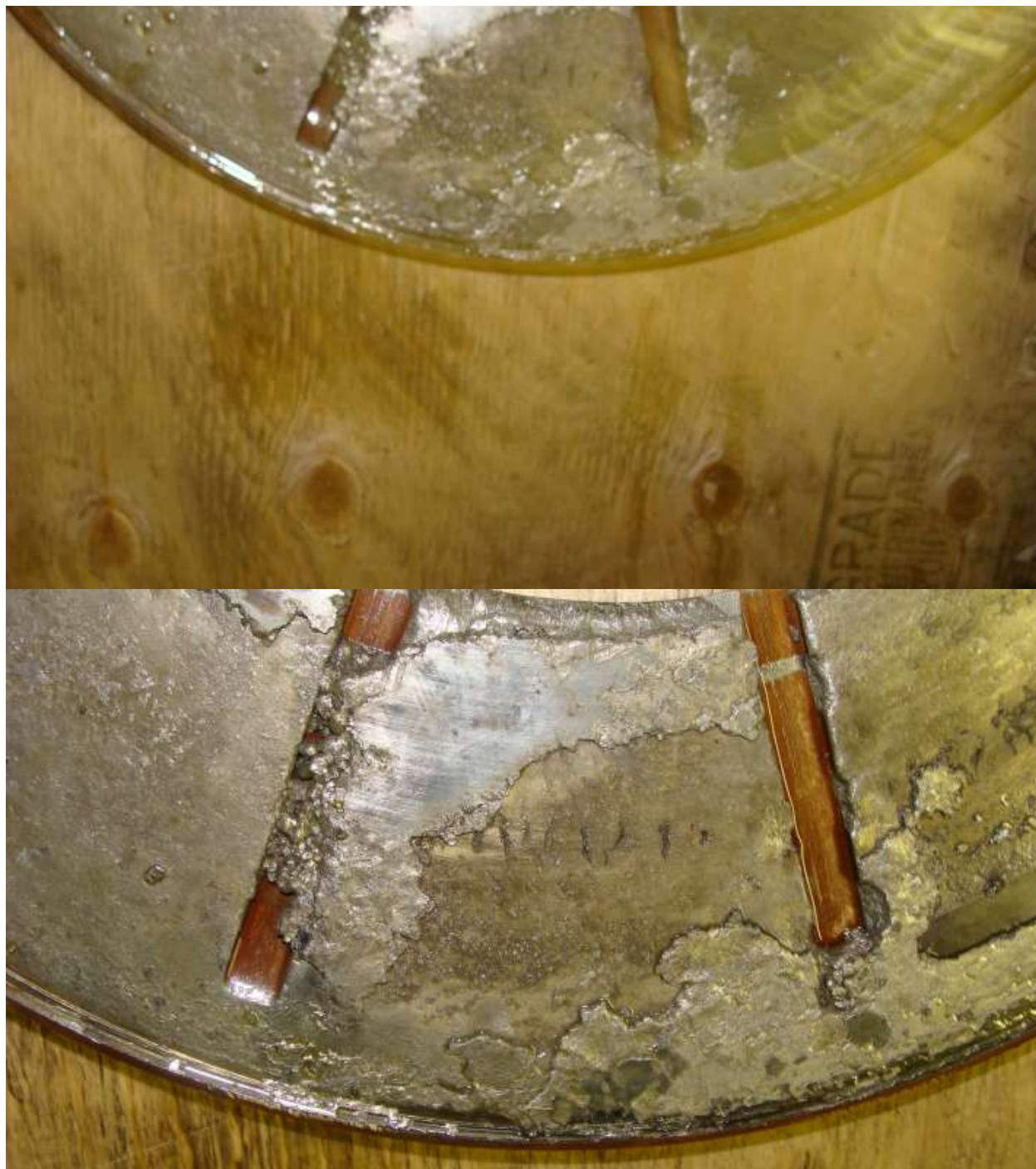
Damage to active side thrust plates
