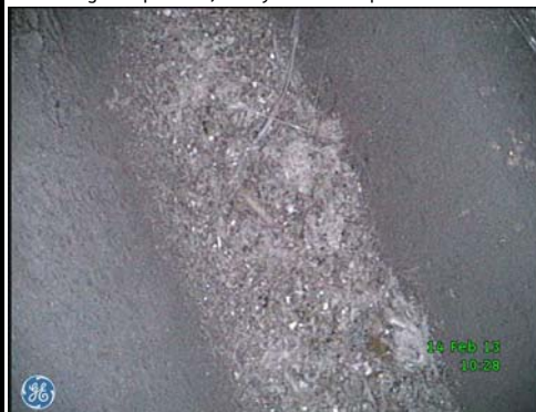
Contamination @ base of stack of coil 1.
