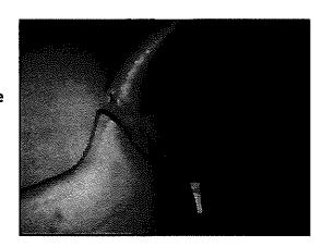
Figure 3: Cracked Discharge Nozzie Bracket
