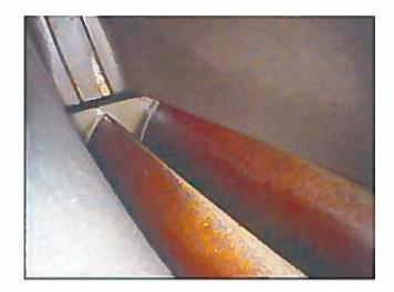
Figure 3: Corrosion on End B Engine
