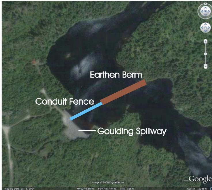
Figure 5 – Proposed fence and berm
