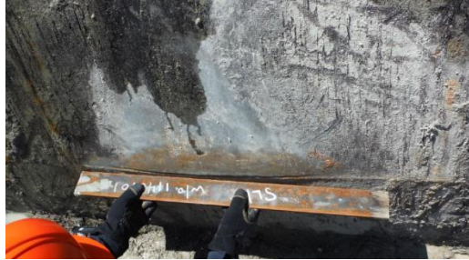
Figure 3-2: Longitudinal Weld Failure Showing Peaking
